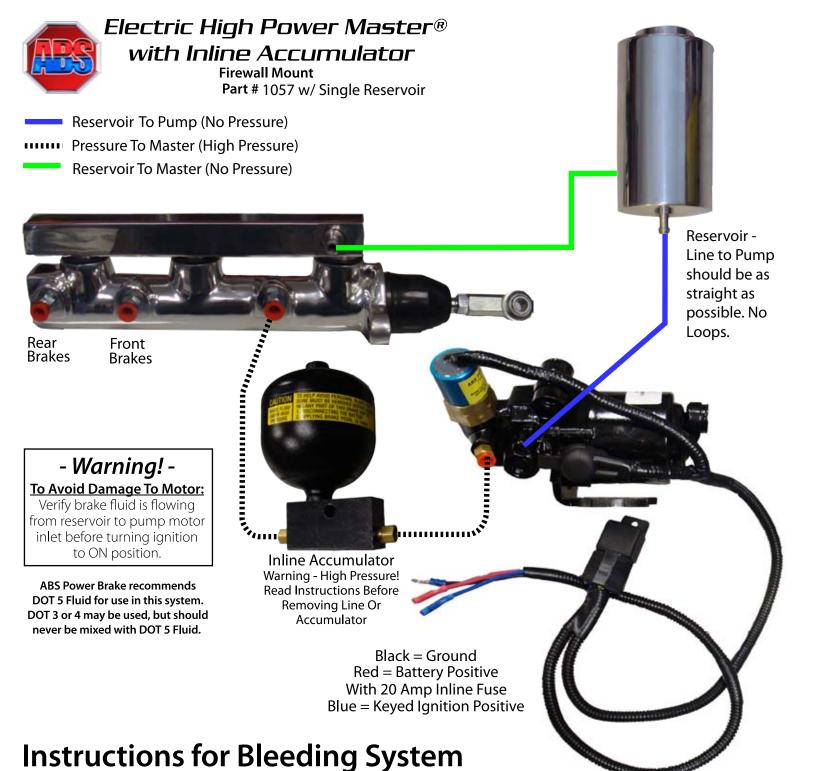
Setup for initial bleeding: It takes two people, one to operate the brake pedal and the other at the bleeder on the wheel cylinder or caliper. The person operating the bleeder should give instructions to the person who is operating the pedal. Bleeder is opened only when the pedal is pushed
